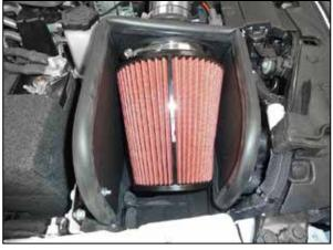
12. Install the air filter onto the filter adapter and secure with the provided hose clamp.
