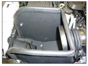
10. Install the heat shield so the mounting studs insert into the mounting grommets and secure to the rubber mounted stud with the provided hardware.
