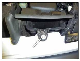
4. Remove the bolt that secures the factory air box to the fender and remove assembly from the vehicle.
