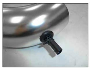
7. Using the provided grommet, install the factory Inlet air temperature sensor into the intake tube.
